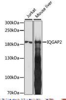
Western blot analysis of extracts of various cell lines, using IQGAP2 antibody (CAB15392) at 1:1000 dilution. Secondary antibody: HRP Goat Anti-Rabbit IgG (H+L) (CABS014) at 1:10000 dilution. Lysates/proteins: 25ug per lane. Blocking buffer: 3% nonfat dry milk in TBST. Detection: ECL Basic Kit (CABM00020). Exposure time: 15s.
