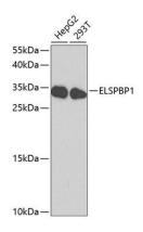
Western blot analysis of extracts of various cell lines, using ELSPBP1 antibody (CAB2151) at 1:1000 dilution. Secondary antibody: HRP Goat Anti-Rabbit IgG (H+L) (CABS014) at 1:10000 dilution. Lysates/proteins: 25ug per lane. Blocking buffer: 3% nonfat dry milk in TBST. Detection: ECL Basic Kit (CABM00020). Exposure time: 90s.
