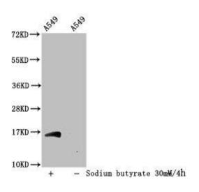
Western Blot. Detected samples: A549 whole cell lysate; Untreated (-) or treated (+) with 30mM sodium butyrate for 4h. All lanes: HIST1H3A antibody at 1:100. Secondary. Goat polyclonal to rabbit IgG at 1/50000 dilution. Predicted band size: 16 kDa. Observed band size: 16 kDa.
