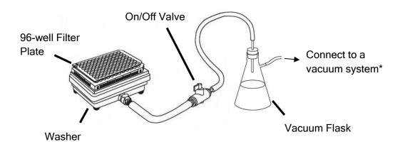
Figure 1: Assay Genie GeniePlex Filter Plate Washer Setup
