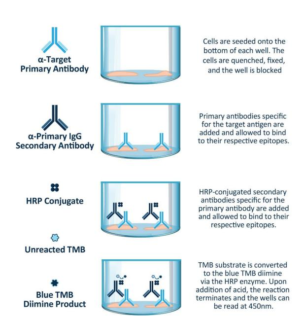
Figure 1. Colorimetric Cell-Based ELISA principle
