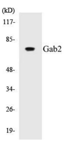
Figure 2. Western blot analysis of extracts from Jurkat cells, treated with TNF 2500U/ml 30', using Gab2 (Ab-623) Antibody.
