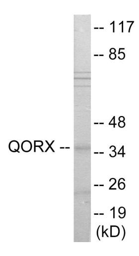
Figure 2. Western blot analysis of extracts from 293 cells, using QORX Antibody. The lane on the right is treated with the synthesized peptide.
