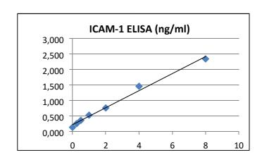
**Note**; curve shown above should not be used to determine results. Every laboratory must produce a standard curve for each set of microwell strips assayed.
