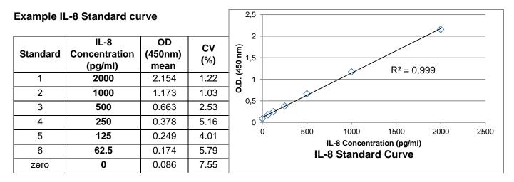
**Note:** curve shown above should not be used to determine results. Every laboratory must produce a standard curve for each set of microwell strips assayed.
