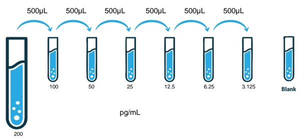
**4. Biotinylated Detection Ab working solution:** Calculate the required amount before the experiment (100µL/well), slightly more than calculated should be prepared. Centrifuge the stock tube before use, dilute the 100× Concentrated Biotinylated Detection Ab to 1×working solution with Biotinylated Detection Ab Diluent.
