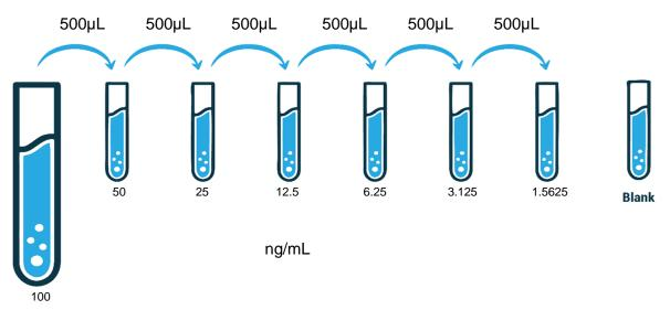
**4. Biotinylated Detection Ab working solution:** Calculate the required amount before the experiment ( $100\mu$ L/well), slightly more than calculated should be prepared. Centrifuge the stock tube before use, dilute the  $100\times$  Concentrated Biotinylated Detection Ab to  $1\times$ working solution with Biotinylated Detection Ab Diluent.
