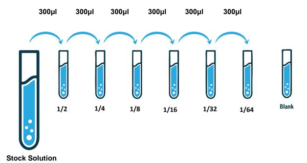
Note: The standard solutions are best used within 2 hours. The standard solution series should be kept at 4°C for up to 12 hours. Or store at -20 °C for up to 48 hours. Avoid repeated freeze-thaw cycles.
