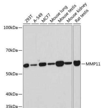
Western blot analysis of various lysates using Rabbit mAb (CAB11088) at 1:1000 dilution. Secondary antibody: HRP-conjugated Goat anti-Rabbit IgG (H+L) (CABS014) at 1:10000 dilution. Lysates/proteins: 25µg per lane. Blocking buffer: 3% nonfat dry milk in TBST. Detection: ECL Basic Kit (AbGn00020). Exposure time: 30s.
