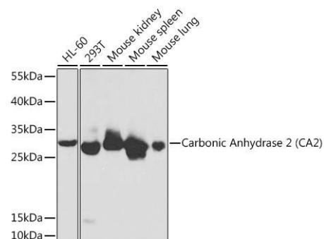
Western blot analysis of various lysates using Carbonic Anhydrase 2 Rabbit pAb (CAB1440) at 1:1000 dilution. Secondary antibody: HRP-conjugated Goat anti-Rabbit IgG (H+L) (CABS014) at 1:10000 dilution. Lysates/proteins: 25µg per lane. Blocking buffer: 3% nonfat dry milk in TBST.
