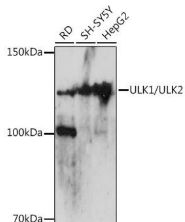
Western blot analysis of various lysates using / Rabbit pAb (CAB18685) at 1:500 dilution. Secondary antibody: HRP-conjugated Goat anti-Rabbit IgG (H+L) (CABS014) at 1:10000 dilution. Lysates/proteins: 25µg per lane. Blocking buffer: 3% nonfat dry milk in TBST. Detection: ECL Basic Kit (AbGn00020). Exposure time: 90s.
