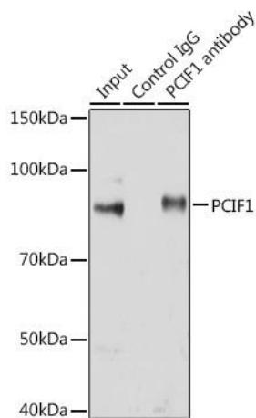
Immunoprecipitation analysis of 200 µg extracts of Jurkat cells using 3 µg PCIF1 antibody (CAB21596). Western blot was performed from the immunoprecipitate using PCIF1 antibody (CAB21596) at a dilution of 1:1000.
