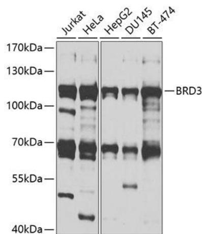
Western blot analysis of various lysates using Rabbit pAb (CAB2277) at 1:1000 dilution. Secondary antibody: HRP-conjugated Goat anti-Rabbit IgG (H+L) (CABS014) at 1:10000 dilution. Lysates/proteins: 25µg per lane. Blocking buffer: 3% nonfat dry milk in TBST. Detection: ECL Basic Kit (AbGn00020). Exposure time: 5s.
