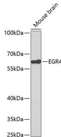
Western blot analysis of lysates from mouse brain, using Rabbit pAb (CAB2910). Secondary antibody: HRP-conjugated Goat anti-Rabbit IgG (H+L) (CABS014) at 1:10000 dilution. Lysates/proteins: 25µg per lane. Blocking buffer: 3% nonfat dry milk in TBST.
