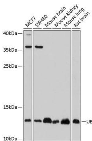
Western blot analysis of various lysates using Rabbit pAb (CAB4028) at 1:1000 dilution. Secondary antibody: HRP-conjugated Goat anti-Rabbit IgG (H+L) (CABS014) at 1:10000 dilution. Lysates/proteins: 25µg per lane. Blocking buffer: 3% nonfat dry milk in TBST. Detection: ECL Basic Kit (AbGn00020). Exposure time: 30s.
