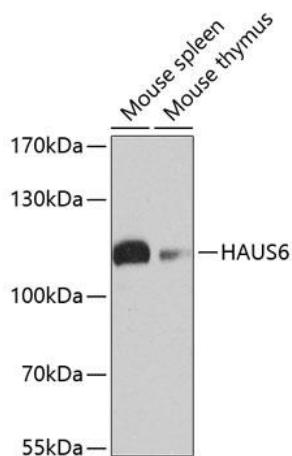
Western blot analysis of various lysates using HAUS6 Rabbit pAb (CAB4797) at 1:1000 dilution. Secondary antibody: HRP-conjugated Goat anti-Rabbit IgG (H+L) (CABS014) at 1:10000 dilution. Lysates/proteins: 25µg per lane. Blocking buffer: 3% nonfat dry milk in TBST. Detection: ECL Basic Kit (AbGn00020). Exposure time: 10s.
