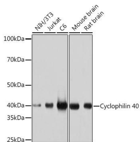
Western blot analysis of various lysates using Cyclophilin 40 Rabbit mAb (CAB5097) at 1:1000 dilution. Secondary antibody: HRP-conjugated Goat anti-Rabbit IgG (H+L) (CABS014) at 1:10000 dilution. Lysates/proteins: 25µg per lane. Blocking buffer: 3% nonfat dry milk in TBST. Detection: ECL Basic Kit (AbGn00020). Exposure time: 10s.
