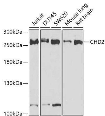
Western blot analysis of various lysates using Rabbit pAb (CAB5895) at 1:1000 dilution. Secondary antibody: HRP-conjugated Goat anti-Rabbit IgG (H+L) (CABS014) at 1:10000 dilution. Lysates/proteins: 25µg per lane. Blocking buffer: 3% nonfat dry milk in TBST. Detection: ECL Basic Kit (AbGn00020). Exposure time: 30s.
