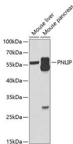
Western blot analysis of various lysates using PNLIP Rabbit pAb (CAB6396) at 1:1000 dilution. Secondary antibody: HRP-conjugated Goat anti-Rabbit IgG (H+L) (CABS014) at 1:10000 dilution. Lysates/proteins: 25µg per lane. Blocking buffer: 3% nonfat dry milk in TBST. Detection: ECL Basic Kit (AbGn00020). Exposure time: 5s.
