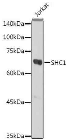
Western blot analysis of lysates from Jurkat cells, using Rabbit pAb (CAB7725) at 1:1000 dilution. Secondary antibody: HRP-conjugated Goat anti-Rabbit IgG (H+L) (CABS014) at 1:10000 dilution. Lysates/proteins: 25µg per lane. Blocking buffer: 3% nonfat dry milk in TBST. Detection: ECL Basic Kit (AbGn00020). Exposure time: 30s.
