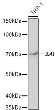
Western blot analysis of lysates from THP-1 cells, using IL4I1 Rabbit pAb (CAB8378) at 1:1000 dilution. Secondary antibody: HRP-conjugated Goat anti-Rabbit IgG (H+L) (CABS014) at 1:10000 dilution. Lysates/proteins: 25µg per lane. Blocking buffer: 3% nonfat dry milk in TBST. Detection: ECL Basic Kit (AbGn00020). Exposure time: 180s.
