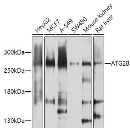
Western blot analysis of various lysates using ATG2B Rabbit pAb (CAB8498) at 1:1000 dilution. Secondary antibody: HRP-conjugated Goat anti-Rabbit IgG (H+L) (CABS014) at 1:10000 dilution. Lysates/proteins: 25µg per lane. Blocking buffer: 3% nonfat dry milk in TBST. Detection: ECL Enhanced Kit (AbGn00021). Exposure time: 60s.
