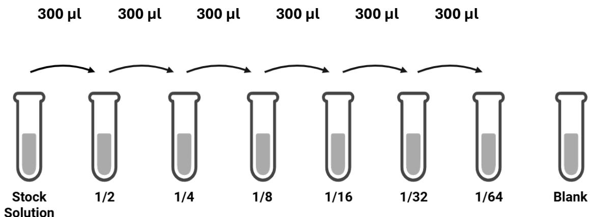
**Note:** The standard solutions are best used within 2 hours. The standard solution series should be kept at  $4^{\circ}\text{C}$  for up to 12 hours. Or store at  $-20^{\circ}\text{C}$  for up to 48 hours. Avoid repeated freeze-thaw cycles.
