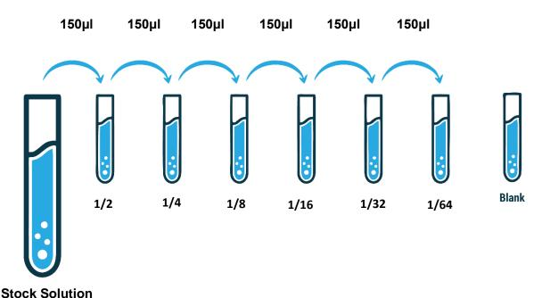
Note: The standard solutions are best used within 2 hours. The standard solution series should be kept at 4°C for up to 12 hours. Or store at -20 °C for up to 48 hours. Avoid repeated freeze-thaw cycles.
