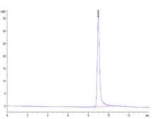
The purity of Cynomolgus IL-17F is greater than 95% as determined by SEC-HPLC.
