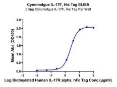
Immobilized Cynomolgus IL-17F, His Tag at  $5\mu g/ml$  (100 $\mu l/well$ ) on the plate. Dose response curve for Biotinylated Human IL-17R alpha, hFc Tag with the EC50 of  $2.4\mu g/ml$  determined by ELISA.
